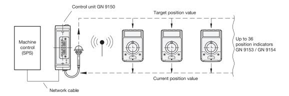
If the target position value and current position value do not match, the LCD display of the position indicator begins to flash. The machine technician must then adjust the position indicator to the correct value. The LCD display shows the difference between the target position value and the current position value and the direction in which it must be turned. It must be turned until a value of 0 appears on the display, meaning zero deviation between the current and target position value.
