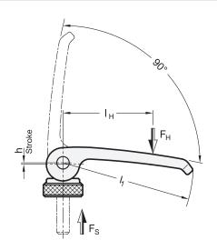
The eccentric principle has two advantages: A large clamping force  $F_{\rm S}$  and a self-locking mechanism as soon as the dead centre is exceeded.
