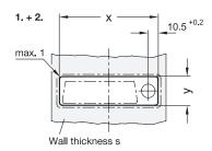
1. The recess in the door for mounting the latch with gripping tray must be cut as shown in the outline drawing.
