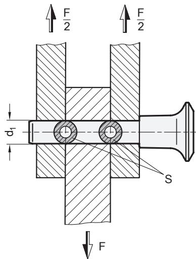
The load capacities specified in the table for the double sided shearing resistance (breaking strength) have been calculated or theoretically defined on the basis of DIN 50141.
