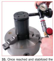
desired pressure, for an easy and safe operation carefully follow the instructions supplied with the charging unit
