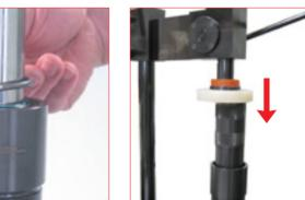
ing C-ring into the groove. When the C-ring enters correctly into the groove you will hear a loud like "CLICK". 49TB... conical centring guide tube.
