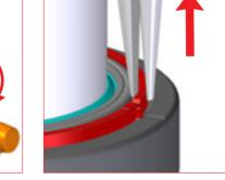
5. By using a rubber mallet, hit the flathead screwdriver to break the OSM ring halfway.
