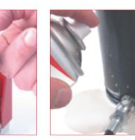
**D.** It is always recommended to check leaks on all connection to and from the cylinder by using the special gas detector 39RFG Special Springs gas detector.
