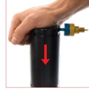
9. Be sure the pressure is completley exhauted by pressing down the piston rod into the cylinder body. Then unthread the discharging device from the discharging hole.
