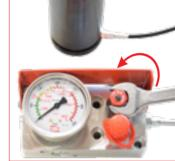
A. To exhaust pressure of hosed cilynders open the discharging valve on the control panel
