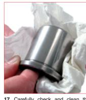
17. Carefully check and clean the piston-rod. If the piston rod shows any damage, wear or scratch do not use it again and replace it with a new one.
