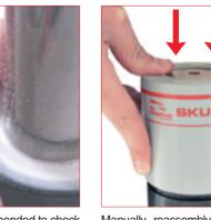
Manually reassembly the protective SKUDO cap on the proper groove on the top of the rod. It would be required a light pressure to correctly position it. When the protective SKUDO cap enter correctly into the groove you will hear a sound like "CLICK".
