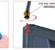
19. Position and thread the one way valve into the hole by using the appropriate special dynamometric tool already calibrated. Torque force required maximum 0.6 Nm. Do not exceed the maximum torque force indicated to not damage the one way valve
