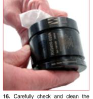
cvlinder body. If the body show any wear or damage do not use it again and replace it with a new one.
