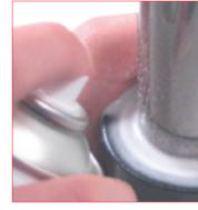
38. It is always recommended to check leaks on the upper side of the cylinders after the maintenance work and before re-using the cylinders by using the special gas detector. 39RFG Special Springs gas detector
