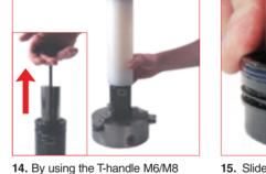
using the proper Screw extracting device (58UT ...) extract the piston-rod and the bush for other models.
