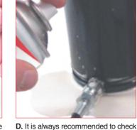
leaks on all connection to and from the cylinder by using the special gas 39RFG Special Springs gas detector
