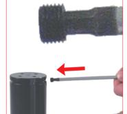
14. By using the hex key (58CE05) thread the one way valve retaining screw 1/8"G (47G1/8G). Pay attention to not tight exessively the retaining screw to avoid damage on the one way valve.
