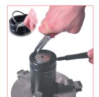
8. By using the removal C-ring (58EAR) and the Multipurpose clamp (58KNIPEX) hook up the retaining C-ring.
