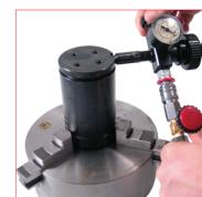
28. Rached and stabilized the desired pressure, for an easy and safety work carefully follow the instructions supplied with the charging unit. 39DMA charging unit.
