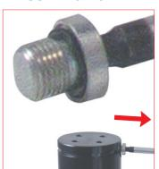
1. Remove the protective screw cap from the charging hole by using the appropriate tool Preserve the the protective screw cap for further reassembly. **58CE05** for the 1/8 G port.
