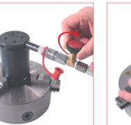
**29.** When directly charging throught **30.** Unthread and relase the the adapter and desired pressure is reached shut off the hose and bottle valves and disconnect the the quick fit coupling.
