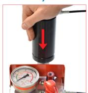
**B.** Be sure the pressure is completley exhausted by pressing down the pis-
