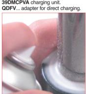
33. Use Special Springs gas detector to check leaks on top of body.
