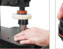
bled bushing into the rod. Be care to position it on the right side, follow the laser print arrows on the bushing.
