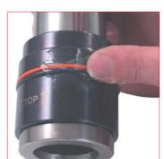
18. Grease the O-ring on the assembled bushing with the specific Special
