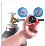
26. Adjust the required maximum pressure trought the regulation valve. The gauge on the right will indicate the maximum allowed pressure to charge the cylinder.
