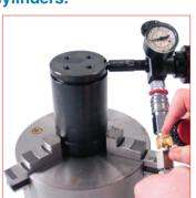
27. Select and assemble the desired charging adapter and thread it on the charging port. For an easy and safety work carefully follow the instructions supplied with the charging unit.
