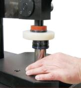
16. Manually or by using the manual press (39PM02A) insert the assem-
