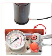
A. To exhaust pressure of hosed cilynders open the discharging valve
