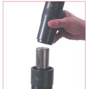
21. Insert the positioning tube over the rod in contact with the upper side of the assembled bushing, then by the manual press, press down into the cylinder body, the piston rod and the assembled bushing. 49TB... conical centring guide tube.
