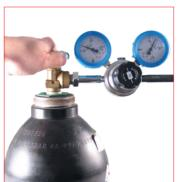
25. Check the correct assembly of the pressare regulation valve on the gas bottle, then open the main tap. The gauge on the left will indicate the bottle pressure.
