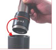
20. Set the positioning tube on the upper part of the cylinder body, then manually insert the piston-rod and the assembled bushing into the position-
