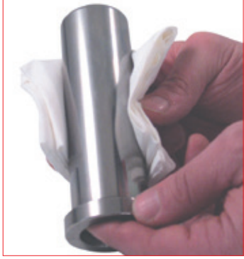
18. Carefully check and clean the piston-rod. If the piston rod shows any damage, wear or scratch do not use it again and replace it with a new one.
