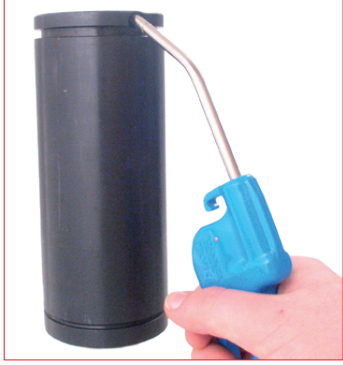
19. Position and thread the one way valve into the hole by using the appropriate special dynamometric tool already calibrated. Torque force required maximum 0,6 Nm. Do not exceed the maximum torque force indicated to not damage the one way valve. 58CD01 dynamometric wrench.
