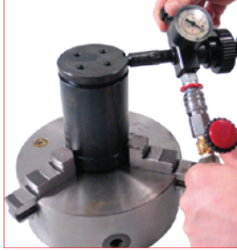
34. Once reached and stabilized the desired pressure, for an easy and safe operation carefully follow the instructions supplied with the charging unit. 39DMA charging unit.
