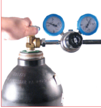
31. Check the correct assembly of the pressure regulation valve on the gas bottle, then open the main tap. The gauge on the left will indicate the bottle pressure. 39R... pressure reducer.
