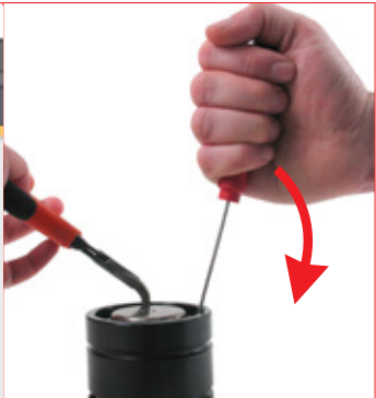
13. By inserting the screwdriver on the appropriate discharging groove, between the retaining ring and the body border, remove the ring as indicated. Use the pliers (58KNIPEX) to avoid that the ring comes out sharply. Use the flat screwdriver 2,5 x 75.
