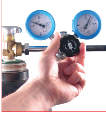
42. Adjust the required pressure on the regulation valve on the bottle. The gauge on the right will indicate the maximum allowed pressure to charge the cylinders. 39R... pressure reducer.
