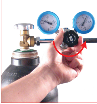
32. Adjust the required maximum pressure through the regulation valve. The gauge on the right will indicate the maximum allowed pressure to charge the cylinder. 39R... pressure reducer.
