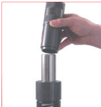
27. Insert the positioning tube over the rod in contact with the upper side of the assembled bushing, then by the manual press, press down into the cylinder body, the piston rod and the assembled bushing. 49TB... conical centring guide tube. 39PM02A manual press.
