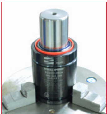
1. Position and clamp the cylinder into a self - centring chuck or a vice .
