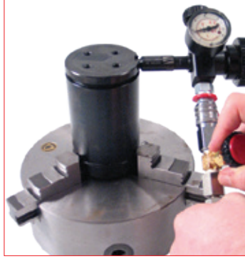
33. Select and assemble the desired charging adapter and thread it on the charging port. For an easy and safe operation carefully follow the instructions supplied with the charging unit. DO NOT exceed the maximum pressure indicated for any specific model. 39DMA charging unit.
