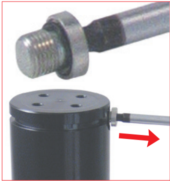
7. Remove the charging plug from the charging hole by using the appropriate tool. Preserve the charging plug for further reassembly. 58CE05 for the 1/8" G port. 58CE03 M6/3 for the M6 port.
