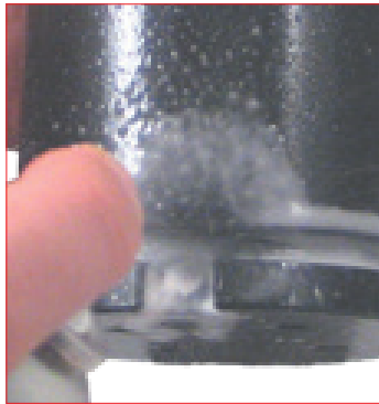
38. It is always recommended to check leaks on the charging port after the maintenance work and before re-using the cylinders by using the special gas detector. 39RFG Special Springs gas detector.
