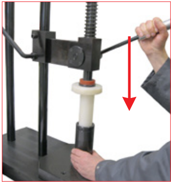
11. Position the anti scratch nylon removal tube (49TN...) on the bush then by the manual press (39PM02A) press all down into the body. The retaining ring is now free for an easy removal.
