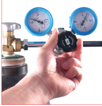
42. Adjust the required pressure on the regulation valve on the bottle. The gauge on the right will indicate the maximum allowed pressure to charge the cylinders. 39R... pressure reducer.
