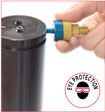
8. Thread DDS discharging device on the charging port then exhaust completely the pressure. Point away from the operator for maximum safety. 39DDS01A BLUE side for M6 hole GOLD side for 1/8"G hole
