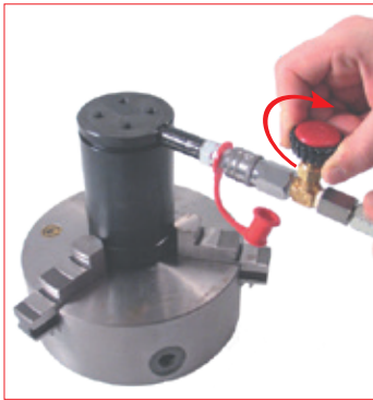
35. When directly charging through the adapter, after the desired pressure is reached, shut off the hose and bottle valves and disconnect the quick fit coupling. For an easy and safe operation carefully follow the instructions supplied with the charging unit. 39DMCPVA charging unit. QDFV... adapter for direct charging.
