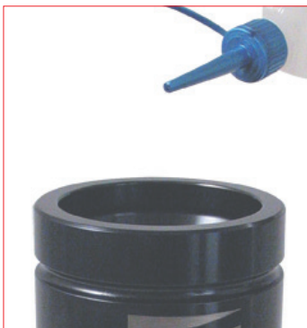
25. Lubricate inside the cylinder body with the specific Special Springs oil supplied with the repair kit. Pay attention to the quantity as indicated for each cylinder model.
