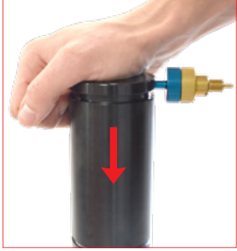
9. Be sure the pressure is completely exhausted by pressing down the piston rod into the cylinder body. Then unthread the discharging device from the discharging hole.
