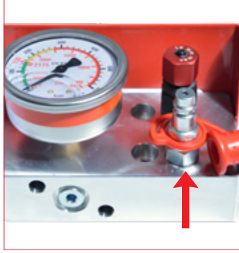
41. After positioning and hosing all the cylinders, proceed through the quick fit device through the control panel for charging all the cylinders. Make sure that the discharging valve is closed properly (15 Nm). 39DMCPVA control panel charging unit.
