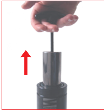
30. Manually extract the assembly piston-rod/bush until it rests against the C-ring. 58EM06 T-handle M6. 58EM08 T-handle M8.
