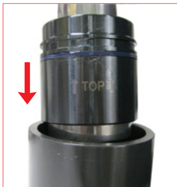
26. Set the positioning tube on the upper part of the cylinder body, then manually insert the piston-rod and the assembled bushing into the positioning tube. 49TB... positioning tube.
