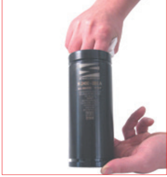
17. Carefully check and clean the cylinder body. If the body show any wear or damage do not use it again and replace it with a new one.
