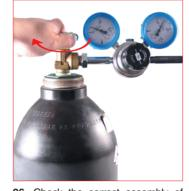
26. Check the correct assembly of the pressare regulation valve on the gas bottle, then open the main tap. The gauge on the left will indicate the bottle pressure. 39R... pressure regulation valve.
