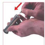
**13.** Carefully clean through the charging hole with an air gun, then drop the new one way valve into the conical hole.
