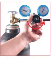
27. Adjust the required maximum pressure trought the regulation valve. The gauge on the right will indicate the maximum allowed pressure to charge the cylinder. 39R... pressure regulation valve.
