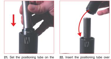
21. Set the positioning tube on the upper part of the cylinder body, then manually insert the piston-rod and the assembled bushing into the positioning tube. 49TB... positioning tube.
