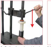
6. Position the anti scratch nylon removal tube on the cartridge (49TN...) then by the manual press (39PM02A) press all down into the body for about 20-25 mm. The retaining ring is now free for an easy removal.
