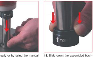
17. Manually or by using the manual press (39PM02A) insert the assembled bushing into the rod. Be care to position it on the right side, follow the
