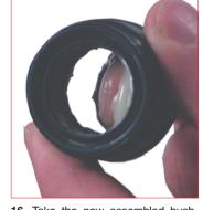
16. Take the new assembled bushing and grease inside all over by using the specific Special Springs grease compound supplied with the repair kit.
