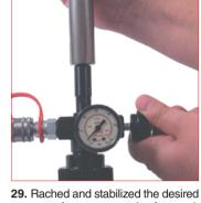
pressure, for an easy and safety work carefully follow the instructions supplied with the charging unit. **39DMA** charging unit.
