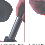
2. Thread the discarging device (DDS-M6/2) on the charging hole then exhaust completley the gas. For safety point the gas flow away from the operator.
