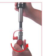
30. When directly charging throught 31. Unthread and relase the the adapter and desired pressure is adapter from the charging hole. charging adapter and thread it on the charging port. For an easy and safety work carefully follow the instructions supplied with the charging unit. DO NOT exceed the maximum pressure indicated for any specific model 39DMA charging unit.
