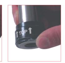
19. Grease the O-ring on the assembled bushing with the specific Special Springs grease compound supplied with the repair kit.
