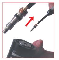
5. Hang and remove the one way valve from the conical lodging site by using the proper tool (39EVU).
